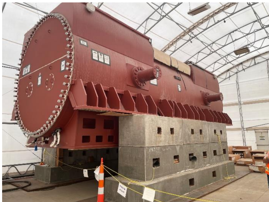
Unit 3 Stator in storage and awaiting installation
